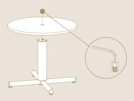
5 Tighten the tabletop by turning the plate clockwise by hand.
