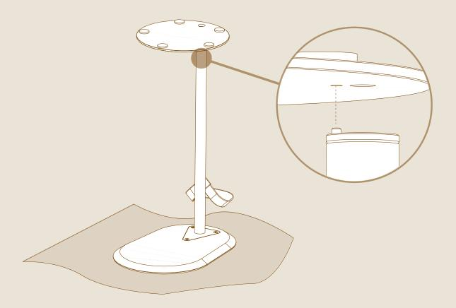
Tighten the M10 screw with its Allen key
