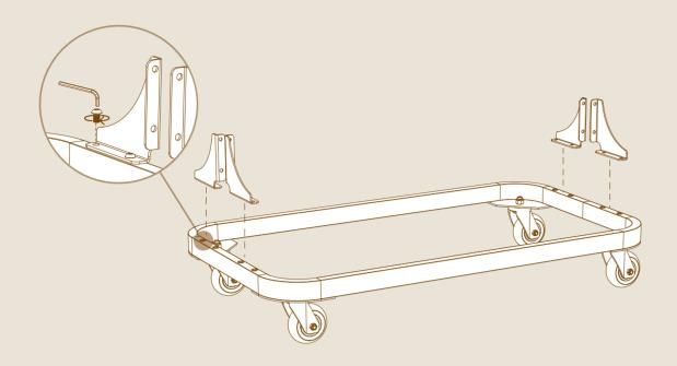
3 Adjust 4 frame angles to the vertical frame.
