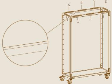
Insert the pins into the selcted holes, first on the top of the Canvas unit and then on the bottom.
