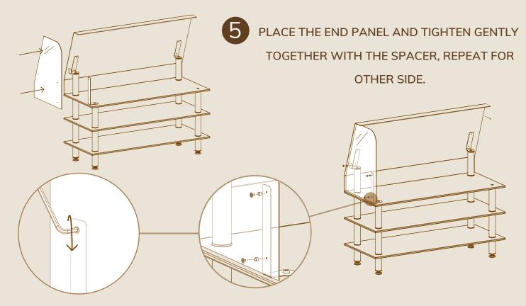
TIGHTEN THE SCREWS ON BOTH SIDES.
