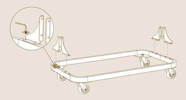
Adjust 4 frame angles to the vertical frame.
