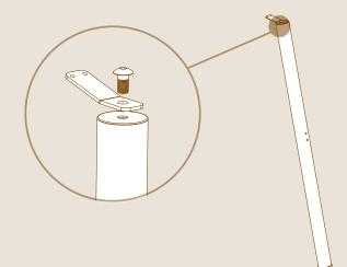
4 Attach the poles to the frame and to the bamboo support arches.
