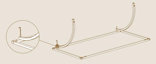
Screw on the angled connectors to the poles, as shown here facing the opposite side of the holes in the pipe.
