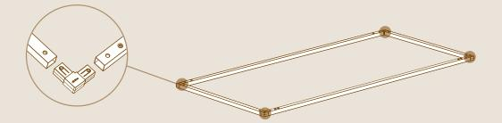
Attach the support arches to the frame on the side with the single hole.
