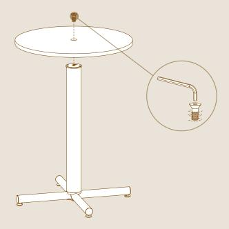
Tighten the tabletop by turning the plate clockwise by hand.
