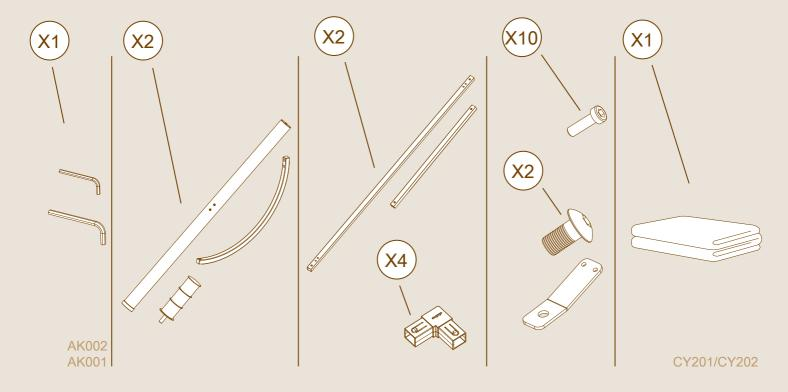
Assemble the frame by clicking the 4 plastic corners.
